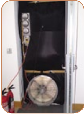
Figure 6.10 Blower door tests involve connecting a fan to a suitable aperture in the building envelope and pressurising it over a range of pressure differences. (Source: ECD Architects)
