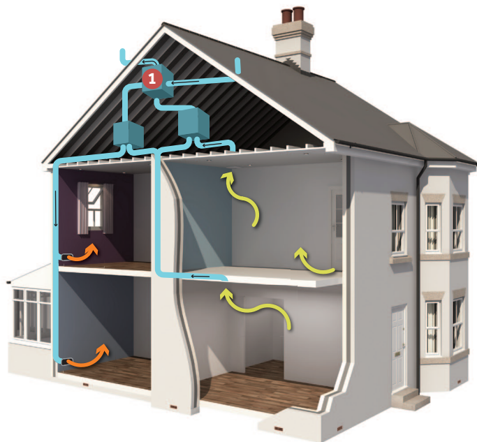
Figure 7.6 Whole-house heat recovery ventilation.
